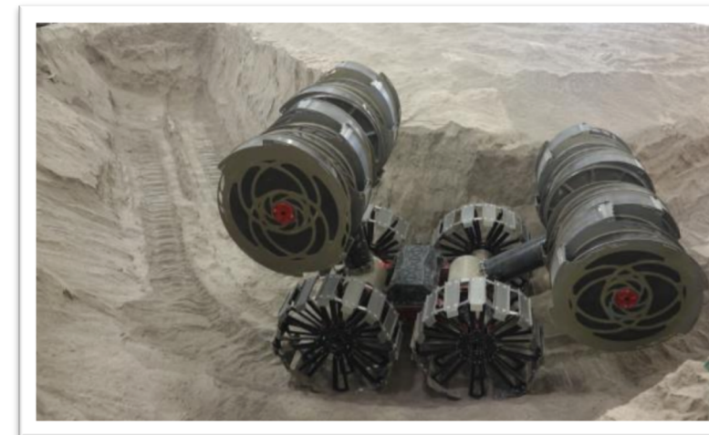
KSC RASSOR excavating a slot trench in BP-1 (Photo Credit – NASA KSC)
